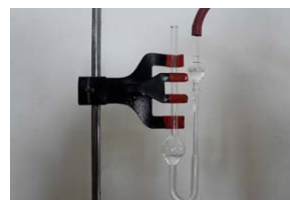
Figure No. 2: Ostwald's Viscometer for measuring Viscosity
