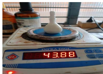
Figure No. 1: specific gravity bottle for the detection of density
