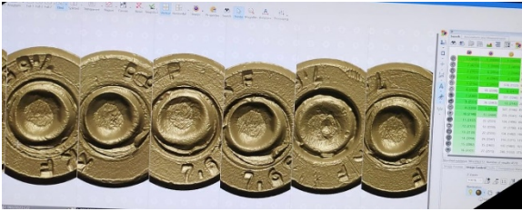
Figure No. 2: Cartridge case examination in Bal-Scan.
